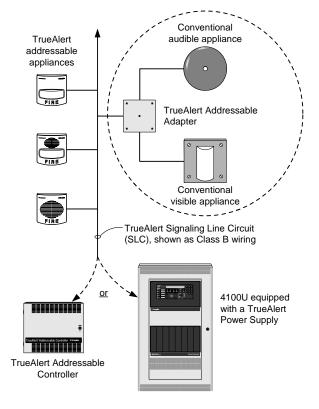
TrueAlert Addressable Adapter Module, Typical One-Line Wiring Reference
